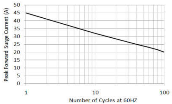
Figure 2. Maximum Non-repetitive Peak Forward Surge Current
